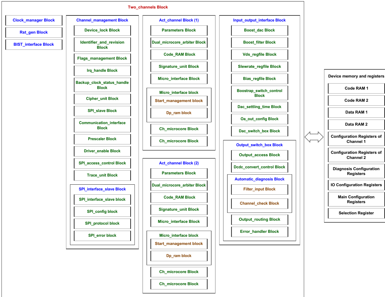
Figure 26. Device logic block hierarchic overview
